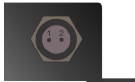
Figure 10: Master Unit back plate power supply pins.
