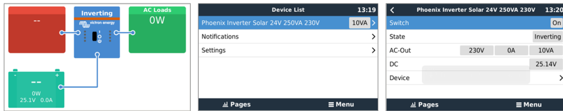
Example of GX screens from left to right: system screen, device list and inverter device screen.
